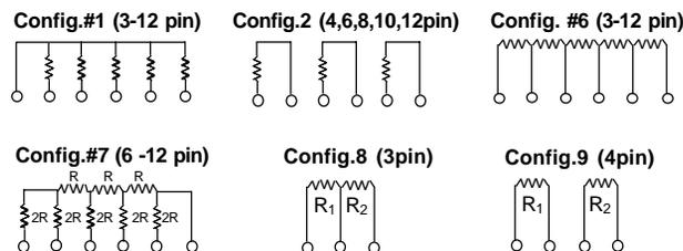
Standard configurations have single resistance value per package except Config's 7, 8, & 9.
